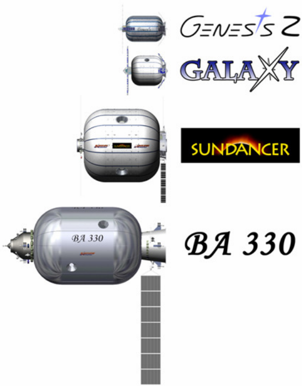
This size comparison between Bigelow Aerospace's future space modules shows that Genesis II is about one-third the size of the first planned human habitable one, Sundancer.
