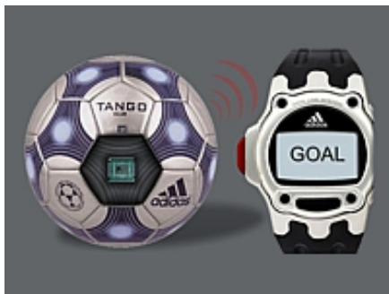
The microchip in the ball relays a signal to a central computer which then sends a message to a watch worn by a referee indicating a goal. http://www.eszak.index.hu
