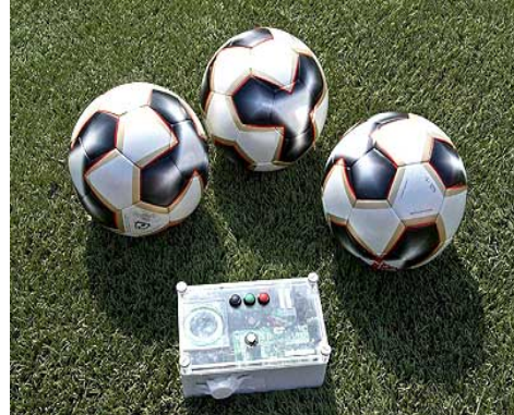
Cairos and Adidas have created a system that places microchips in balls that relays ball position information to a receiver. http://www.geileteile.net
